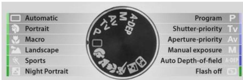
Fig. 1.13: Various basic and advanced photography modes of DSLR cameras
